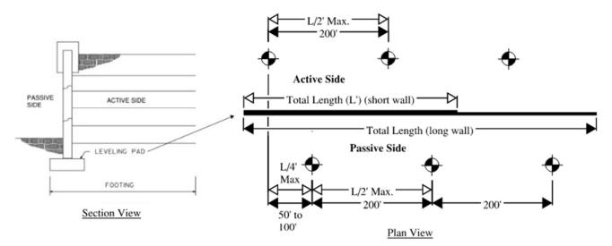
Boring Spacing for Short MSE Walls are those with "L" and white arrows. Boring Spacing for Long MSE Walls are those with numerical values and black arrows; the number of borings for Long MSE Walls is not limited to the six shown in the example above, but should be increased to adequately sample the full length of the wall
